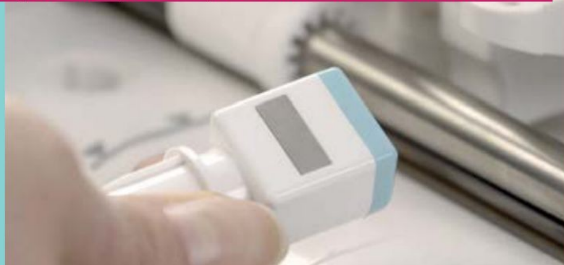
The new Auto Tool Detection feature brings up the required options when a tool is inserted
