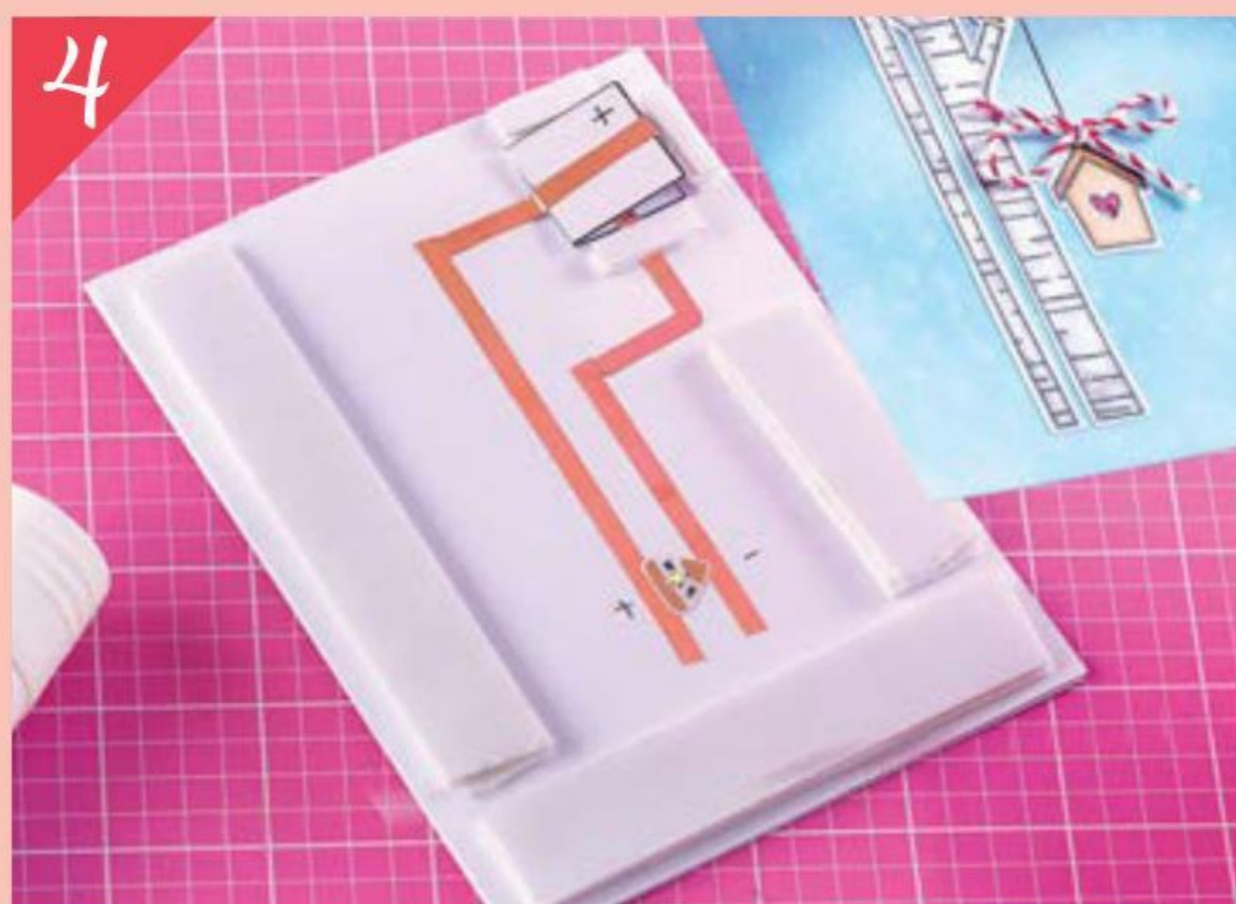
4 Stick the LED light over the mark. Apply three layers of foam tape around the battery to hold it in place
